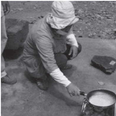
Photo 13: Measuring the water content of a soil mixture
