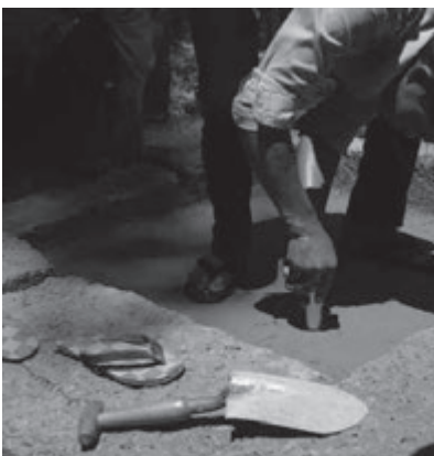
Photo 19: Compaction control using a Yamanaka hardness meter
