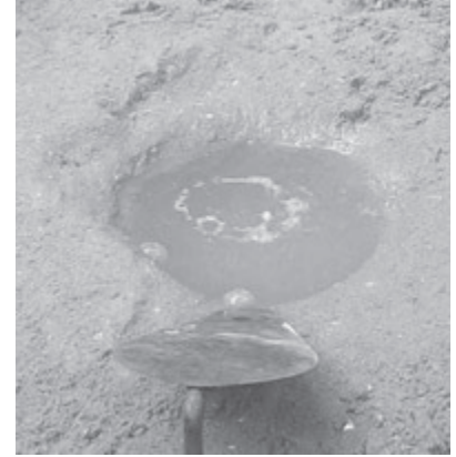
Photo 24: Adding water to a bare hole to see if it can keep its shape
