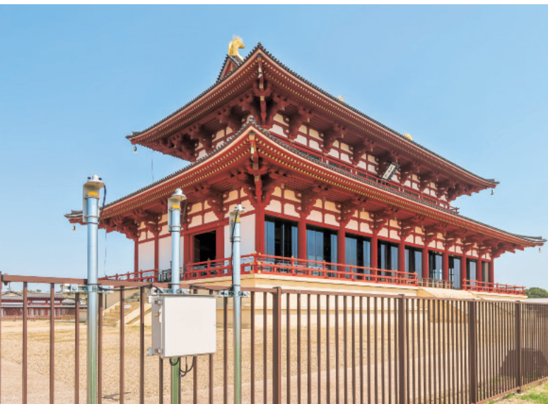
保存修復科学研究室：建造物彩色の劣化の検討のための環境調査 Conservation Science Section: Survey of preservation environment for the examination of deterioration of architectural coloration
