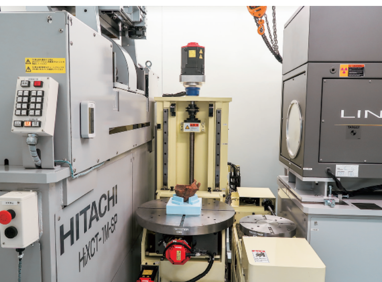
保存修復科学研究室：新設X線CT装置による出土遺物構造調査 Conservation Science Section: Investigation of the structure of recovered artifacts with a newly installed X-ray CT device
